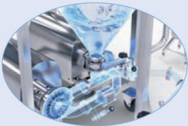
Cleaning liquid is poured into the hopper
